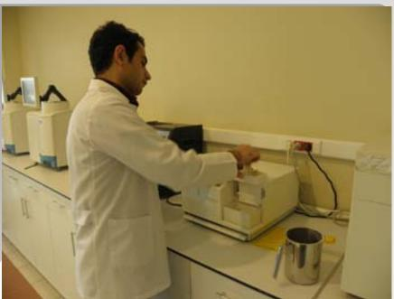
Second, protein and hardness tests are conducted.
