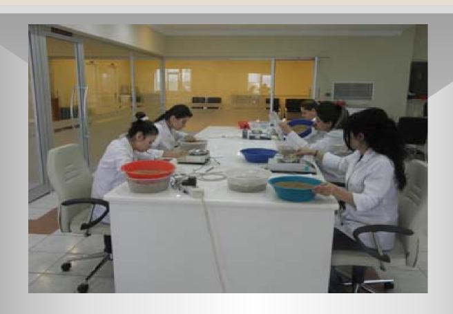
Engineers determine the percentage of damaged and broken kernels, and other grains.
