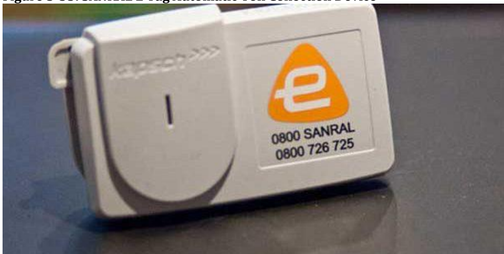
Figure 3-33: SANRAL E Tag Automatic Toll Collection Device
