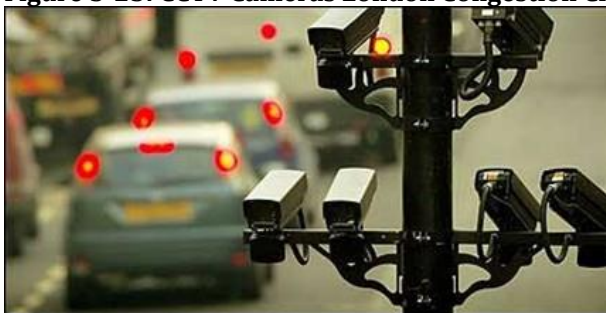
Figure 3-23: CCTV Cameras London Congestion Charging System
